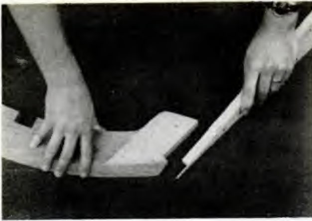
PLANKING-SHEER-CHINE fits into bow-piece notch. Notice plywood members fastened to the underside
